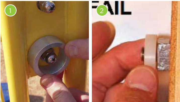
Gauges are used to test the compliance of all projections. This projection is in compliance because it does not extend beyond the face of the gauge. This bolt end is an unsafe protrusion.
